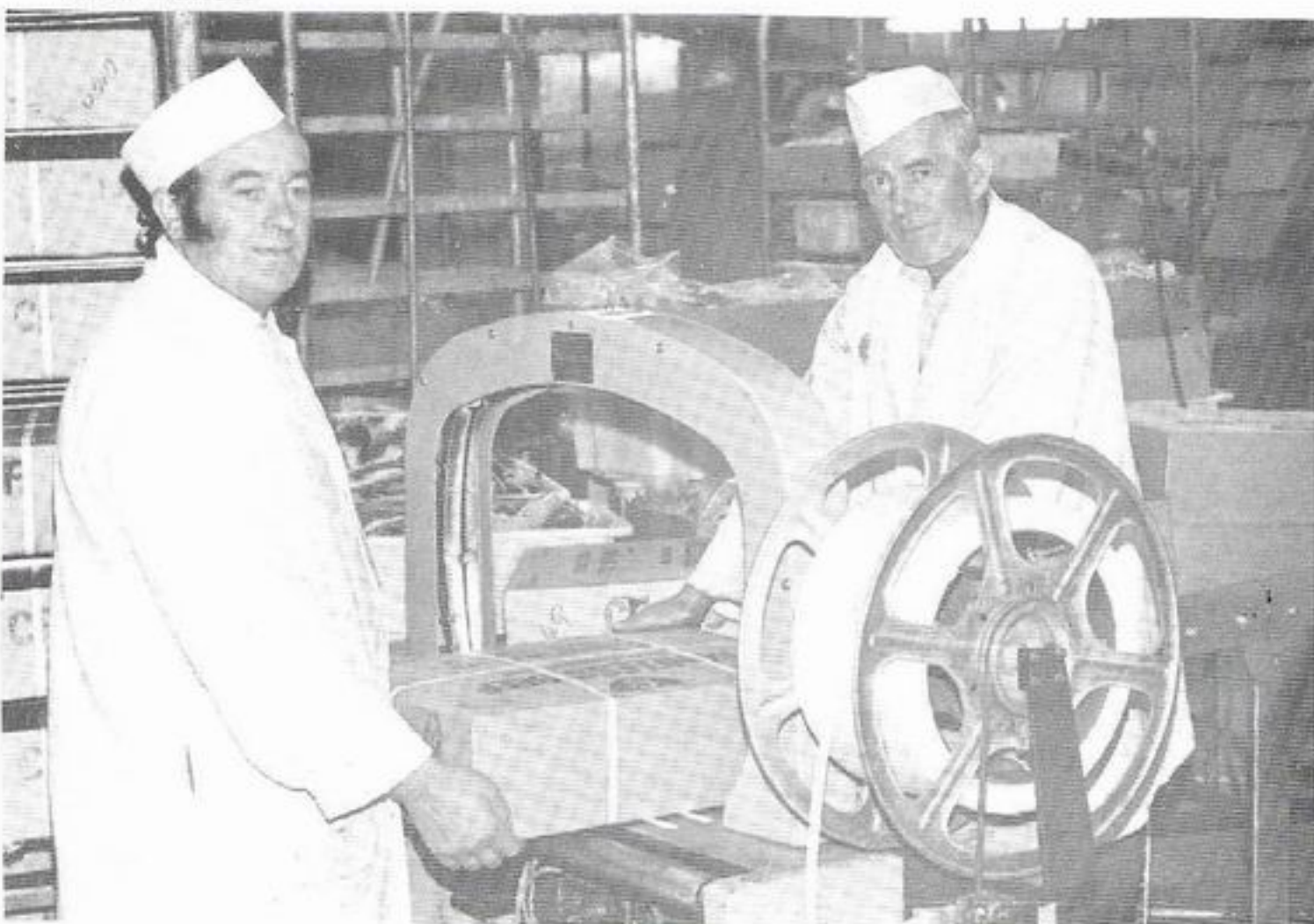
At the end of the line (Boning) Bill Daly and Denny Lynch strapping and "racking" boxes of Boneless Beef.
