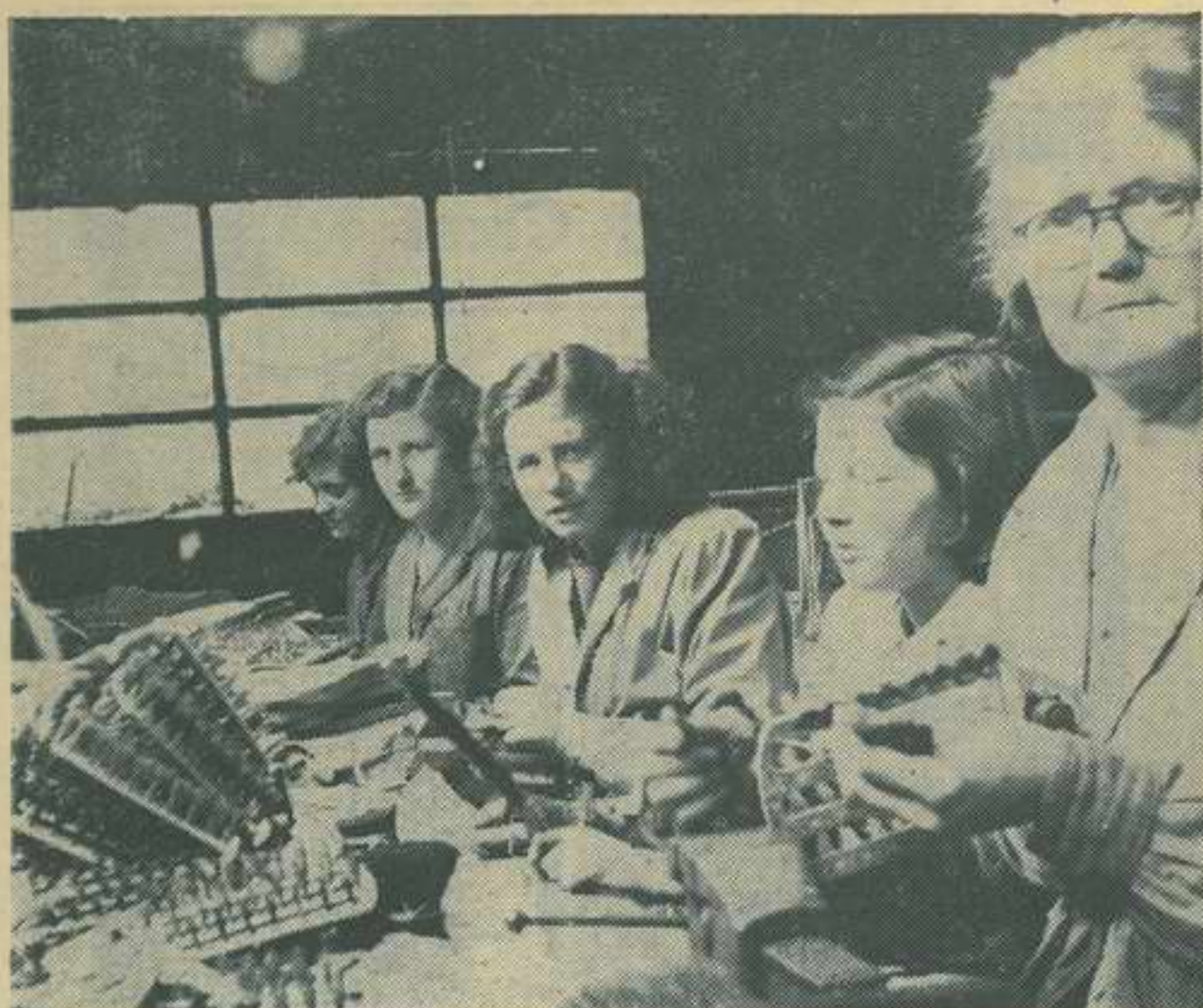
Using one of the oldest and best methods of brush manufacture, these workers are hand-drawing brushes.
