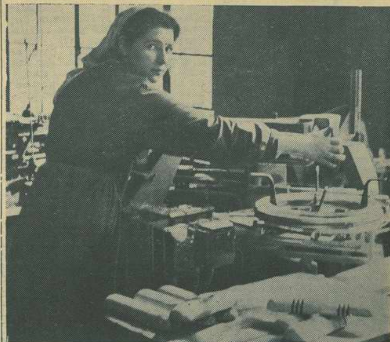
This operator turns out brushes on the brush-filling machine. A comparison of the two photographs on this page emphasis the way in which Varians make use of the best of the old and the new methods of brush making.
